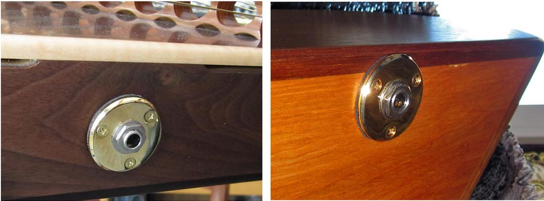
If you choose a bottom mount (as in the picture on the right) there must be enough space below the soundboard for the jack to fit and wires to come out of it without hitting the underside of the soundboard.
